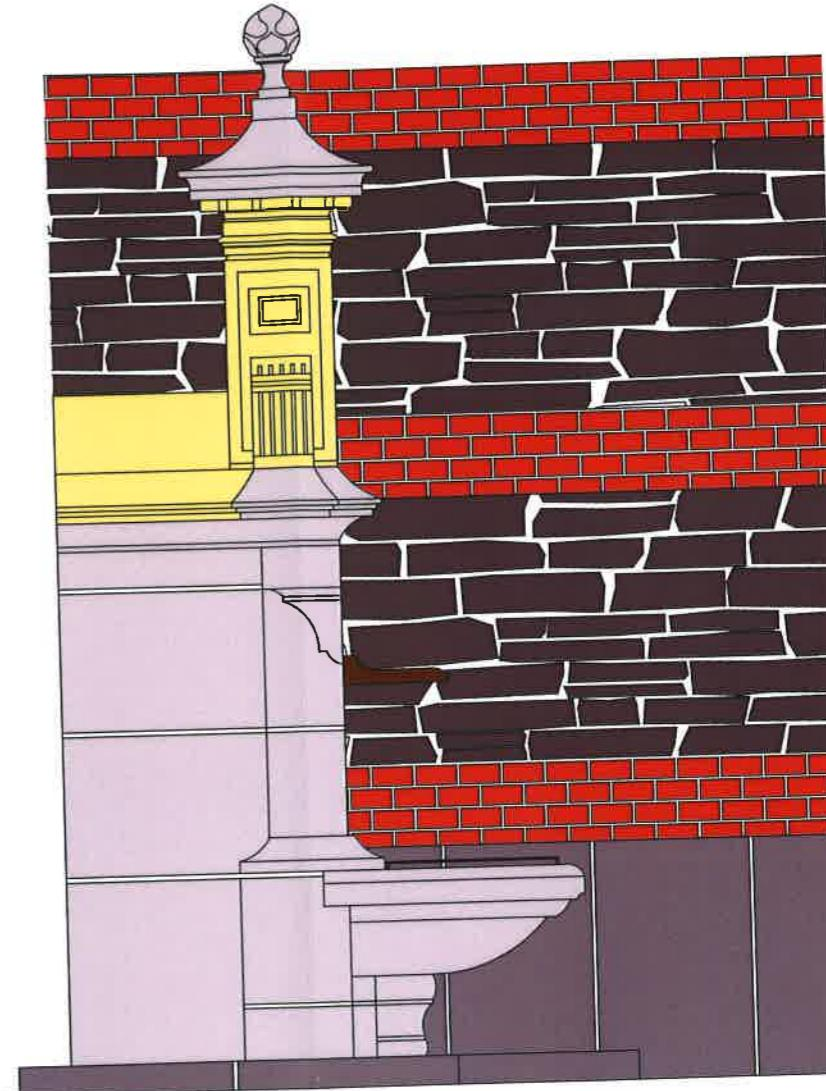
PRVKY ZE ŽULY BUDOU PO OČIŠTĚNÍ DOPLNĚNY RESTAURÁTORSKÝM TMELEM NA HYDRAULICKÉ BÁZI, DŘEVĚNÉ
